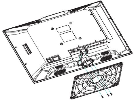
Cover a flat stable surface with a soft cloth. Place the TV unit facedown on the cloth. First align the base with the holes on the back of the unit and fix it with 4 PB4\*14mm screws. Then match the holes in the stand with the fixing pins in the bottom of the base. Fasten with 3 BB3\*8mm screws.
