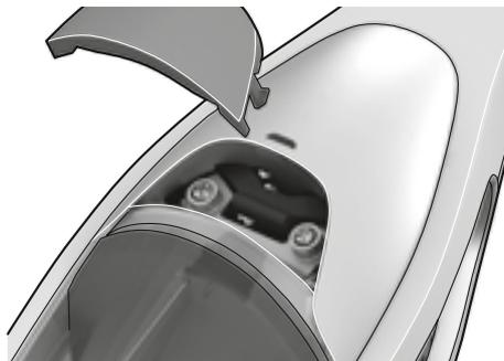
2. Release the button and carefully lift the hood.
