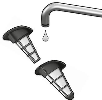
**4. Separate filters.** Shake them clean or rinse separately using warm water. Make sure filters are dry before reassembling in reverse order.
