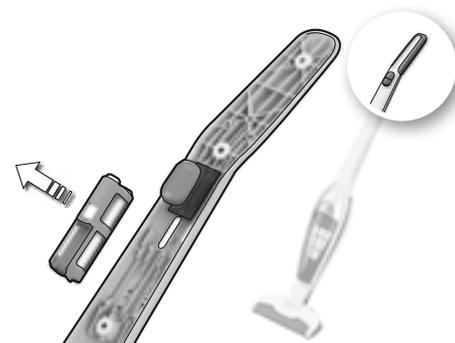
3a. Unclip the connecting cables and lift out the batteries. Batteries should be removed from the appliance before it is scrapped.
