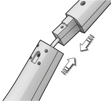
**1. Fit the handle by carefully inserting it into the lower main body.** Make sure that the cable does not jam.
