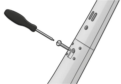
**2. Secure the handle** by tightening the locking screw supplied. Use a screwdriver or a coin.
