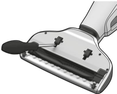
1. If the wheels need to be cleaned, remove them carefully by using a small screwdriver.
