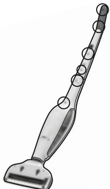
1. Run batteries flat and disconnect UniRapido from the charging station. Undo the 11 screws (2 of them hidden under the release button).
