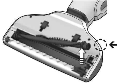
1. Push the brush roll release button. The hatch cover will come slightly free and the brush roll can now be removed.
