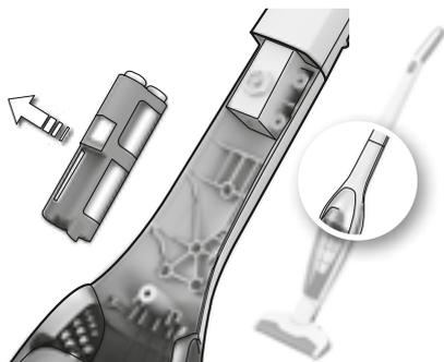
3b. Unclip the connecting cables and lift out the batteries. Batteries should be removed from the appliance before it is scrapped.
