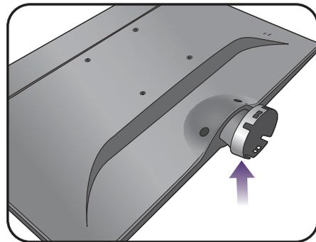
Orient and align the stand base socket with the end of the stand arm, then push them together until they click and lock into place.
