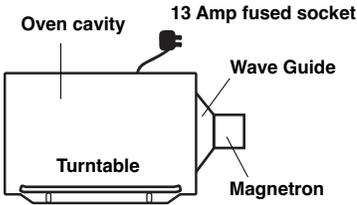
In a microwave oven, electricity is converted into microwaves by the MAGNETRON
