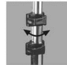
1. Take out rod set and against slide hose hanger. Install the hanger.
