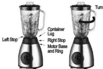
1. To tighten container bottom, put assembled container securely into motor base ring with handle and lug in front of the right stop.
