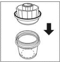
Place mill on motor housing. Support mill and switch on to grind.
