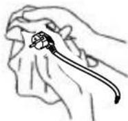
A build-up of dust on the plug will attract condensation, which could cause cable damage resulting in fire.
