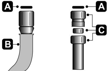
**Connection with steel hose:** Use only continuous wall steel hoses which comply with the relevant regulations, and always fit the provided gasket **A** between the hob fitting and the hose itself **B**.
