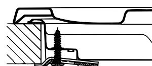
Hooking position for top  $H=30 \text{ mm}$
