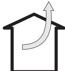
In the extractor mode air is discharged to the outside by a special conduit. In that setting any charcoal filters shall be removed (see page 20).
