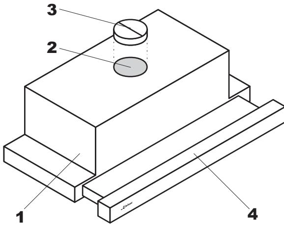
1. Hood body, equipped with lights, engines unit and electronic programmable control.
